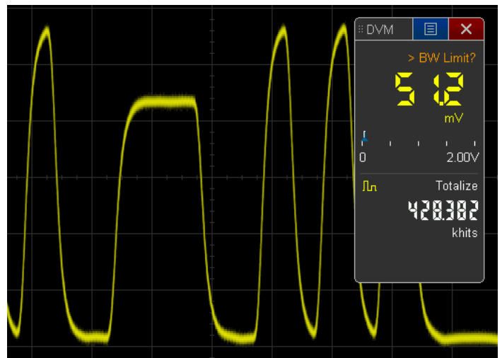
Figure 35. Totalizing the number of runt errors.
