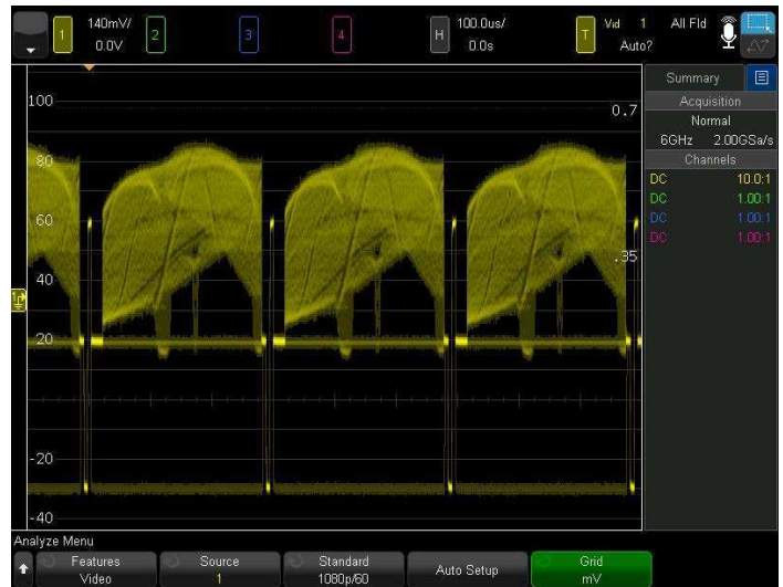
Figure 45. Triggering on a 1080p/60 signal.
