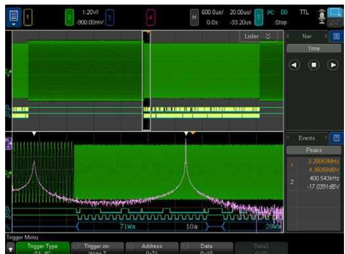
Figure 37b. Gated FFT time correlating the FSK frequency hopping with an I 2 C command (write 7 @ 0x71 data 10).
