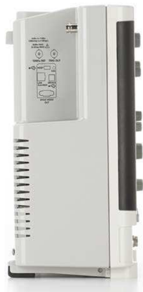
Figure 8. One- gigahertz-per-inch form factor: 6 GHz, 6 inches deep.
