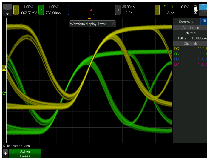
Figure 54. Quick Freeze Display preserves the persistence.
