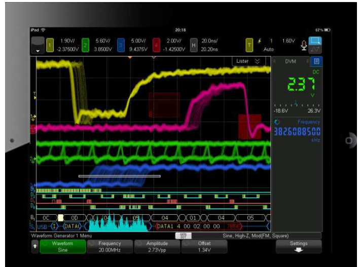
Figure 53. Controlling the 6000 X-Series via tablet device.
